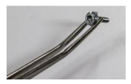
It can be challenging to install small screws in tight places. Instead of clumsy fingers in a slender fuselage, a great way to hold and guide small parts is with curved-tip tweezers. For maximum versatility, the tweezers' tip should be rounded and as close to 90 degrees as possible. Also use the tweezers to grip small parts to avoid losing them as you remove them from tight spots
