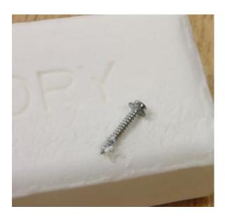
Wood screws don't always thread in as effortlessly as we'd like; it can be hard on your hands and the model. Next time, try swiping the screw's threads across a damp or dry bar of soap. The soap acts as a lubricant, making it much easier to thread the screw in. It is particularly useful in tight areas where it is difficult to get a good grip on tools.
