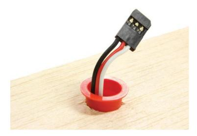
At one time or another, most of us have had to fish for a servo extension wire that slipped back inside the wing; but there is a solution. Cut a 3/16-inch hole in the bottom of the red plug from an old bottle of epoxy. Across the hole, cut a slot that's just wide enough to squeeze the connector at the end of your servo extension through. Trim the access hole in the wing to fit the plug, and you'll never have to go fishing again. This trick also works well for hold-down bolts.
